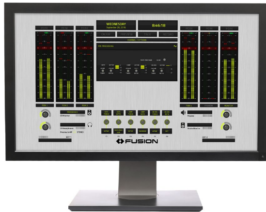
Channel Mic processing view with VU meter ballistics shown
